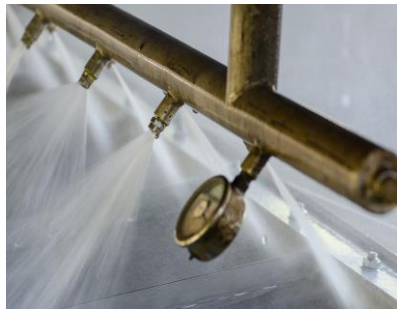
Pressure cleaning the filter mesh
