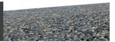
**Artificial washed gravel** is produced by grinding larger fractions of natural siliceous aggregate from the Zuera gravel pit, which are is screened and washed.
