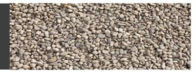
**Coarse aggregate** that undergoes double washing and classification; basically siliceous composition, round with no fines or organic material.
